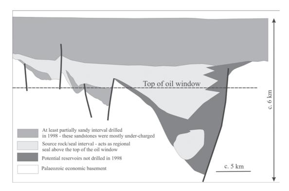
Fig. 2. Schematic W-E cross-section across the North Falkland Basin, illustrating the under-charged sands above the regional source-seal couplet, and untested marginal sands (darkest shading). (See Fig. I for approximate profile location).
