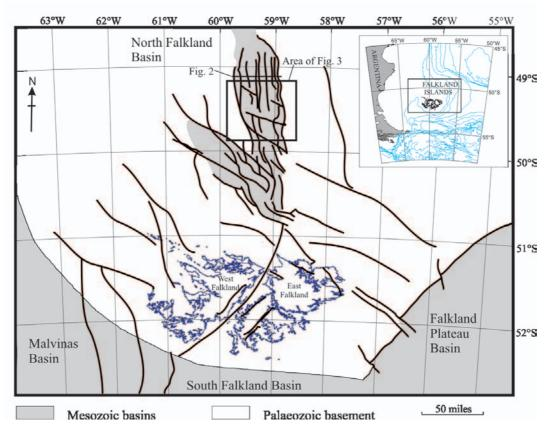
Fig. I. Outline map of the Falklands basins and the controlling fault trends. Jurassic-Cretaceous extensional faults in the North Falkland Basin are oriented north-south. The NW-SE oriented lineaments reflect an underlying and reactivated Palaeozoic structural grain. Box shows the location of Fig. 3. The Mesozoic basins (grey shading) are surrounded by a Palaeozoic platform (white).
