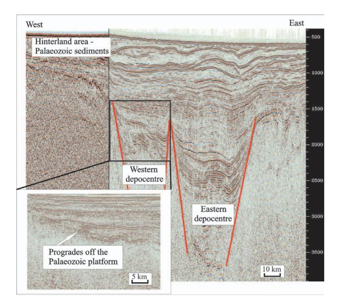
Fig. 5. West-east composite seismic section across the North Falkland Basin, illustrating the platform area that forms the hinterland for the fans (vertical scale is in ms TWT). The inset box shows detail of an Early Cretaceous delta complex prograding off the platform into the western depocentre of the North Falkland Basin.
