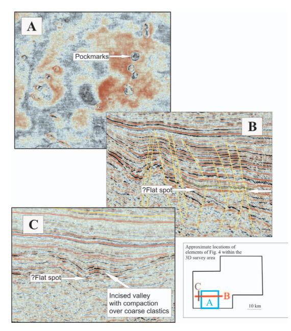
Fig. 4. Seismic panels from the new 3D dataset in the North Falkland Basin, showing: (a) horizontal slice illustrating pock-marks at approximately 650 ms TWT; (b) flat spot at 2500 ms TWT in the Liz fan area; (c) flat spot at the base of convex-up channel fill sandstones within the feeder to the Liz fan.
