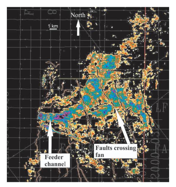
Fig. 8. "StratAmp" display of the Liz fan. The background amplitudes from the lacustrine claystones have been masked with a black marker band in this display in order to highlight the shape and intensity of the amplitudes over the Liz fan.
