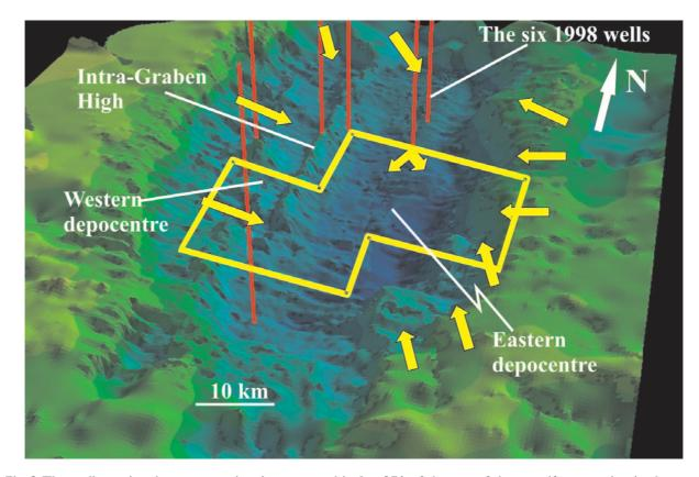
Fig. 3. Three-dimensional representation (constructed in Arc 3D) of the top of the syn-rift succession in the central part of the North Falkland Basin, based on 1997 and older 2D seismic data, showing fault offsets, relay ramps and transfer zones, which are the predicted sand entry points to the basin (yellow arrows) and the new 3D survey area (yellow box). The positions of the 1998 wells are shown as red lines. See Fig. 1 for location.
