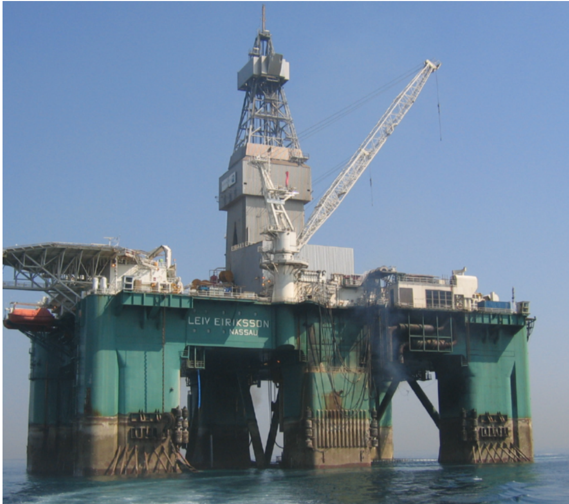
Figure 4.1. The Ocean Rig 'Leiv Eiriksson DP semi-submersible rig' (Appendix A)
