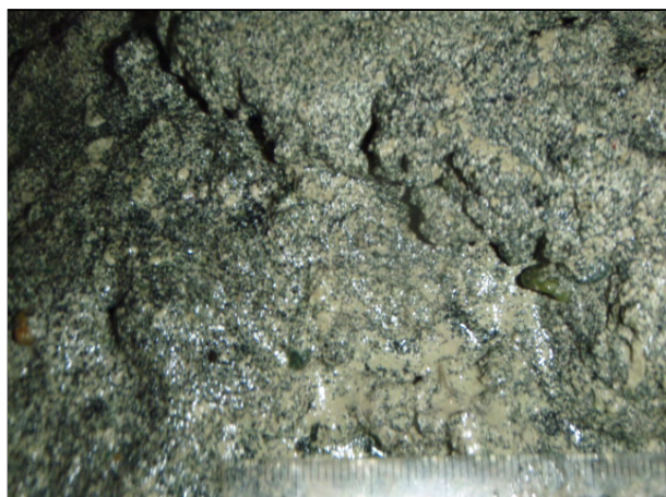
Easting: 868 805 m Depth: 1436 m Northing: 4 323 434 m Sed Type: Silty sand with dark sandy patches
