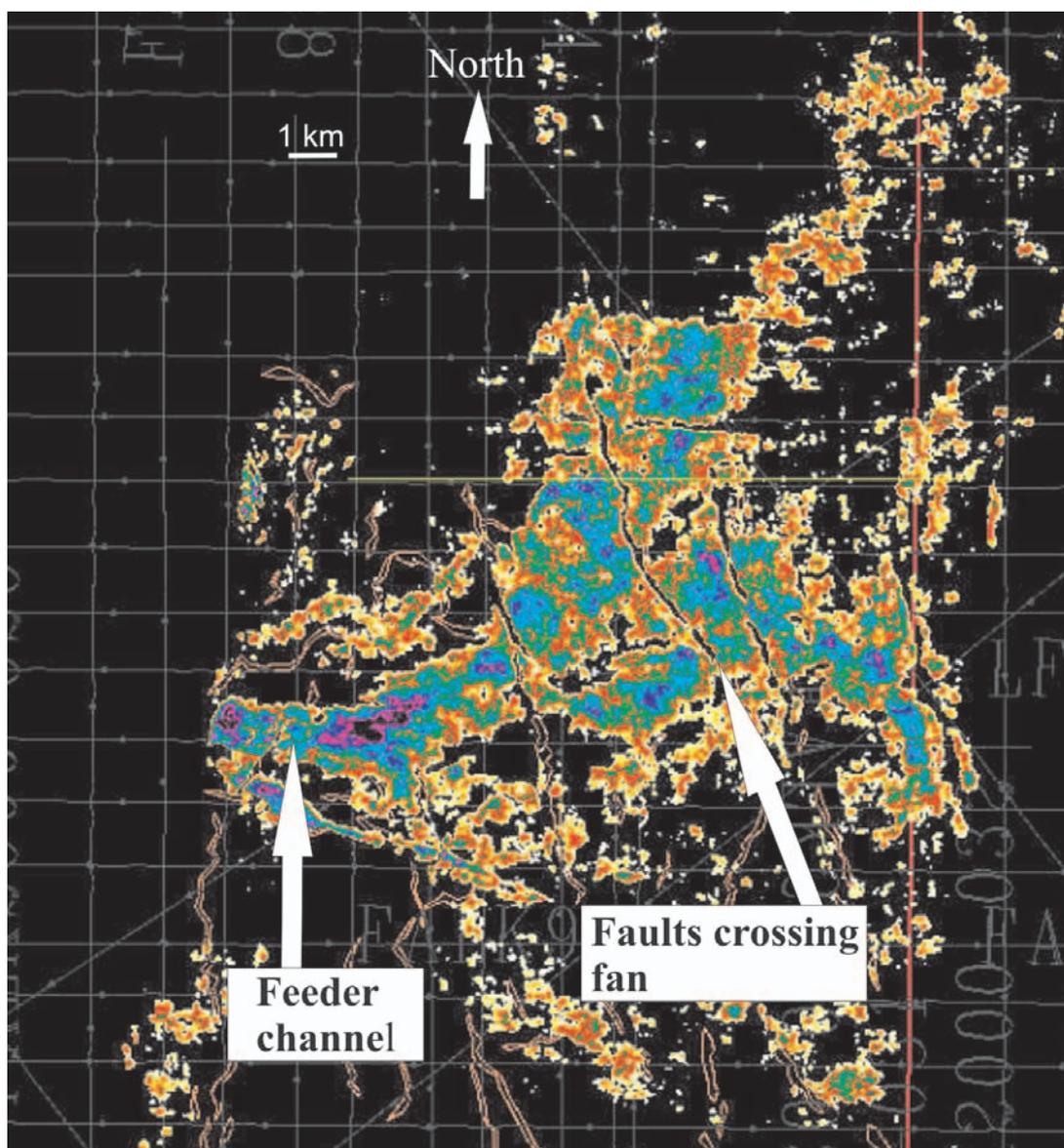
**Fig. 8.** “StratAmp” display of the Liz fan. The background amplitudes from the lacustrine claystones have been masked with a black marker band in this display in order to highlight the shape and intensity of the amplitudes over the Liz fan.
