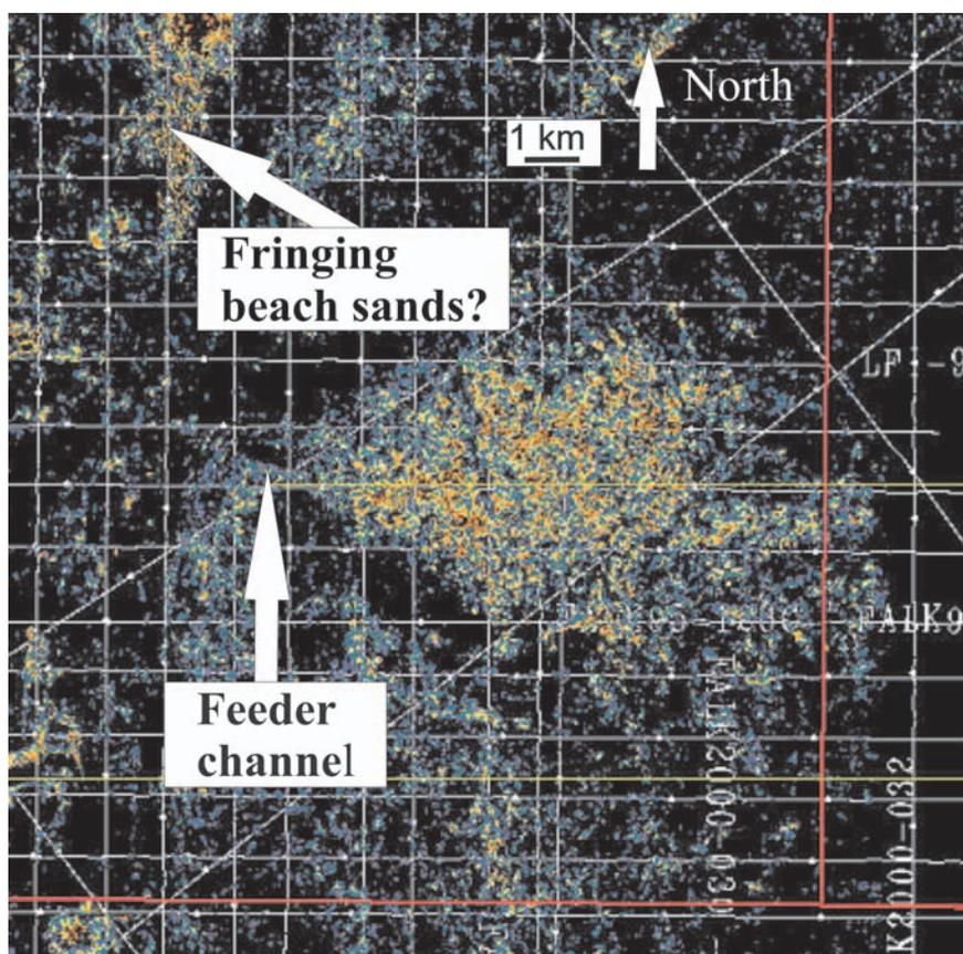
**Fig. 9. “StratAmp” display of the Beth fan. The background amplitudes from the lacustrine claystones have been masked with a black marker band in this display in order to highlight the shape and intensity of the amplitudes over the Beth fan.**
