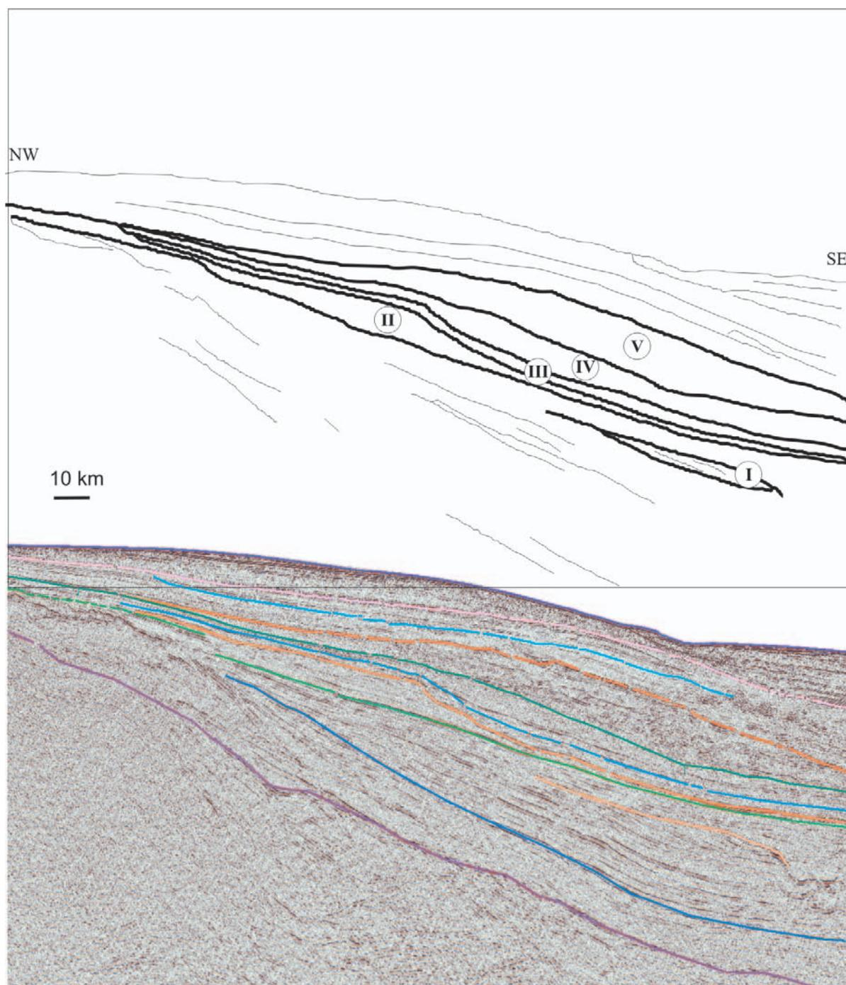
**Fig. 12. Seismic section (and line drawing) oriented NW-SE across the western margin of the Falkland Plateau Basin, illustrating individual fans labelled I to V. Seismic acquired by Western-Geco, 1993.**
