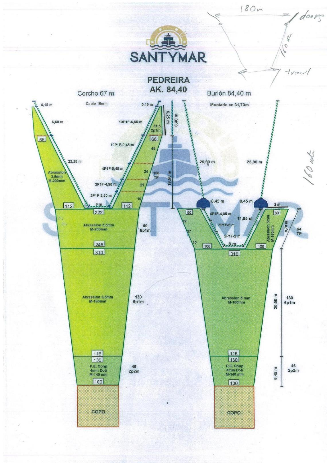
Figure A1. Schematic and measurements of the bottom trawl used during the research survey.
