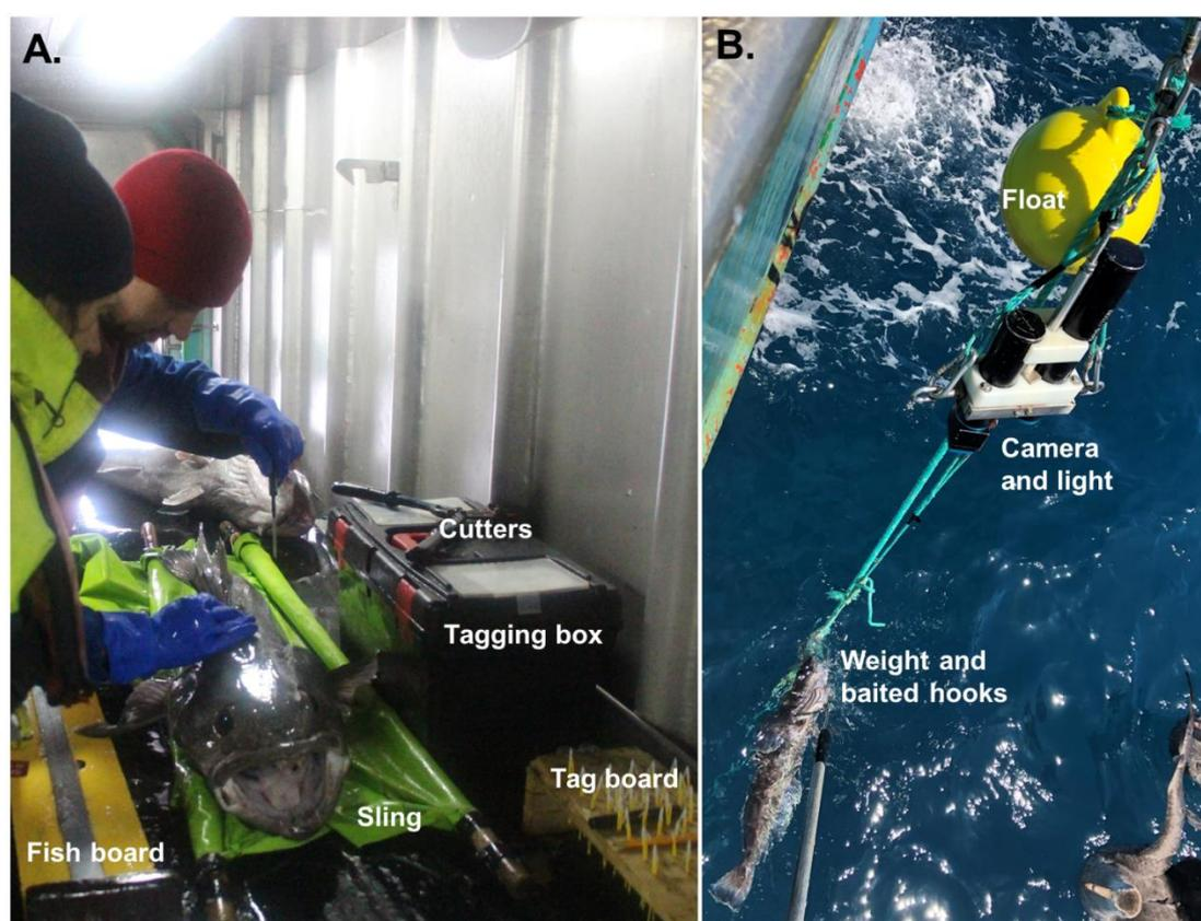
**Figure 2. Tagging station and camera set ups.** A. Layout of the tagging station showing the location of the fish measuring board, cutters, fish sling, tagging box and tag holding board. B. Set-up for the camera deployment showing the arrangement of the weight, baited hooks, camera, and float. This set-up corresponds to the schematic in Figure 3.
