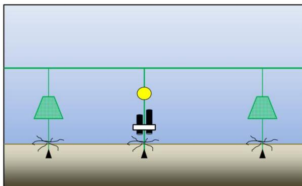
**Figure 3. Camera deployment configuration during the November 2018 research cruise.** All 8 deployments were conducted with no umbrellas and the camera pointing down towards the baited hooks and seabed.
