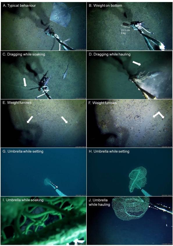
**Figure 9. Stills from the camera footage showing behaviour of the fishing gear.** The weight and bait behaviours are shown during typical soaking (A), when slightly slack due to current (B), slowly dragging due to current (C), and dragging rapidly while hauling (D). The weight being hauled created furrows in the seabed (E, F, white arrows). The behaviour of the umbrella is shown while setting (G, H), soaking (I), and hauling (J).
