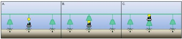
**Figure 4. Camera deployment configurations during the February 2018 research cruise.** The first 8 deployments were be conducted with no umbrellas (A), the 9<sup>th</sup> deployment was conducted with the umbrella above the camera (B), and the last two deployments were condcuted with the camera above the umbrella (C).
