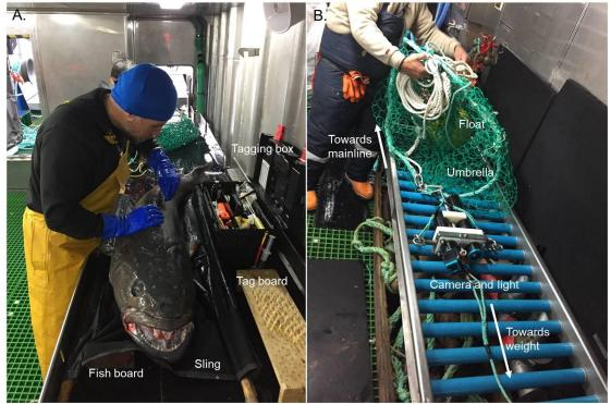
**Figure 3. Tagging station and camera set ups.** A. Layout of the tagging station showing the location of the fish measuring board, fish sling, tagging box and tag holding board. B. Set-up for the camera deployment showing the arrangement of the weight, camera, umbrella, and float. This set-up corresponds to the schematic in Figure 4C.
