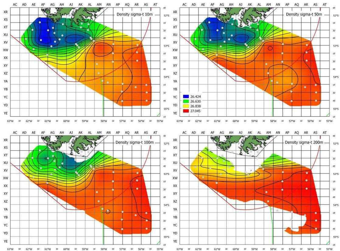
**Figure 43: Density at 10m, 50m, 100m and 200m (contours at 0.05 sigma-t)**
