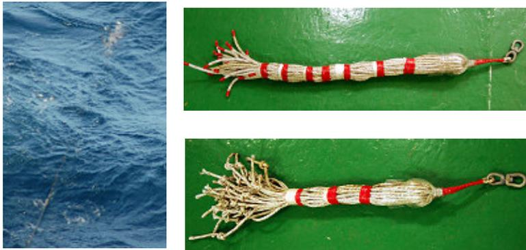
Figure 33: Experimental tension devices tested on *Dorada*.
