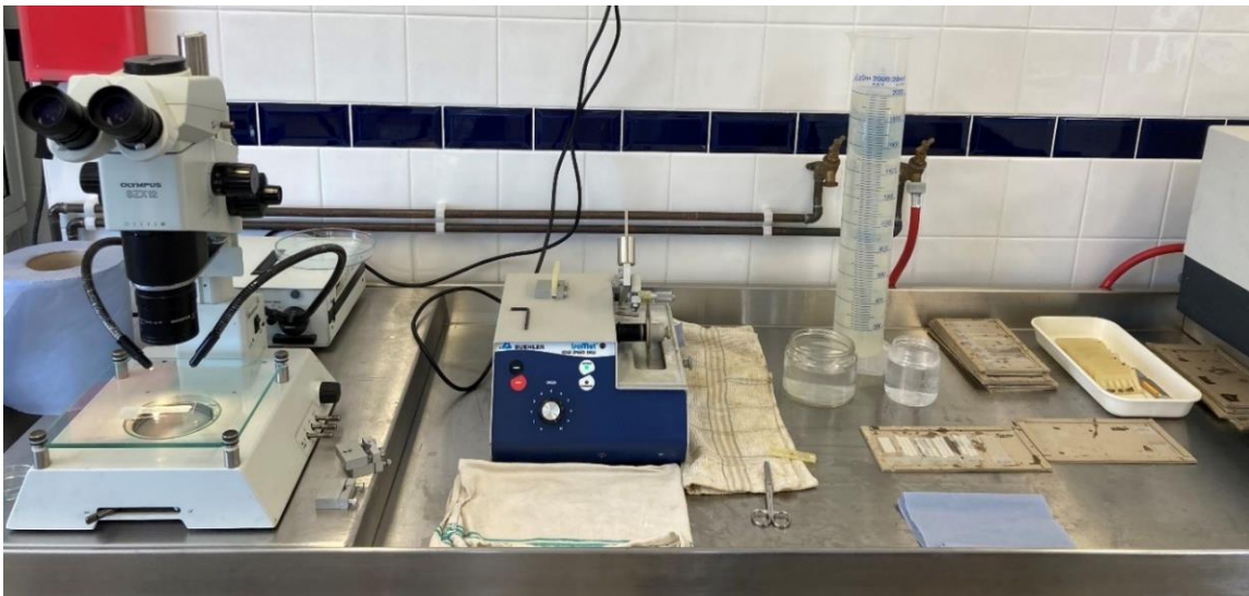
Figure 7. Set up of the cutting area with BUEHLER IsoMet® Low Speed Saw, dissecting microscope and all the needed materials.
