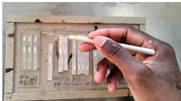
Figure 9. Embedded sections on a microscope slide (on the left) and sections waiting to be embedded (on the right).
