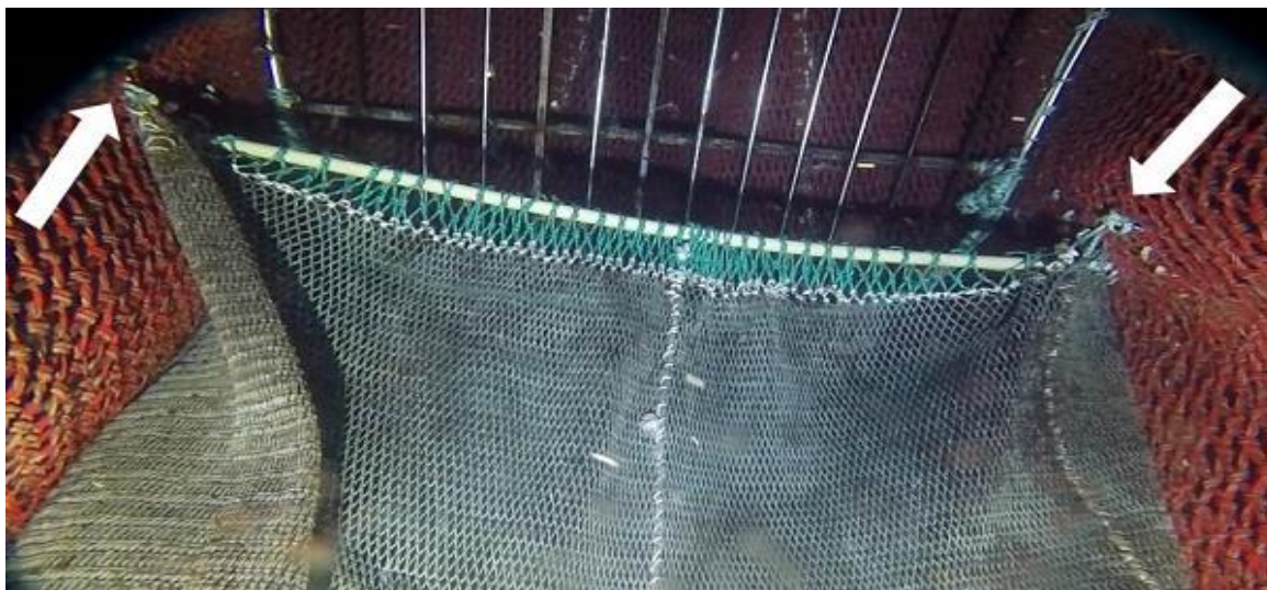
Fig.7. Compliant SED-B. The arrows indicate the attachment of the small mesh panel to the sides of the net. The internal escape hole is neither blocked by ropes nor mesh. Note the PVC tube in the border of the panel.
