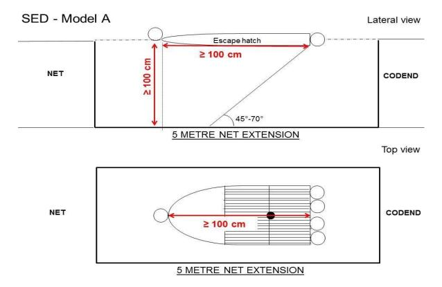
**Fig.2.** Lateral and top view of SED-A.
