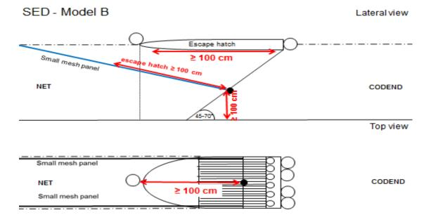
Fig.4. Lateral and top view of SED-B.
