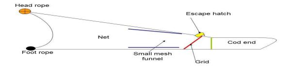
Fig.5. General diagram SED-C.
