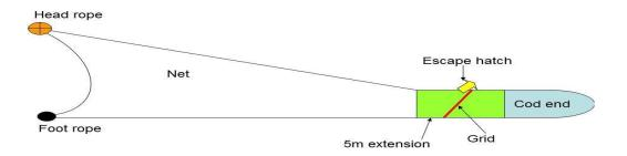
Fig.1. General diagram SED-A with 5 m net extension
