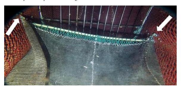
**Fig.7.** Compliant SED-B. The arrows indicate the attachment of the small mesh panel to the sides of the net. The internal escape hole is neither blocked by ropes nor mesh. Note the PVC tube in the
