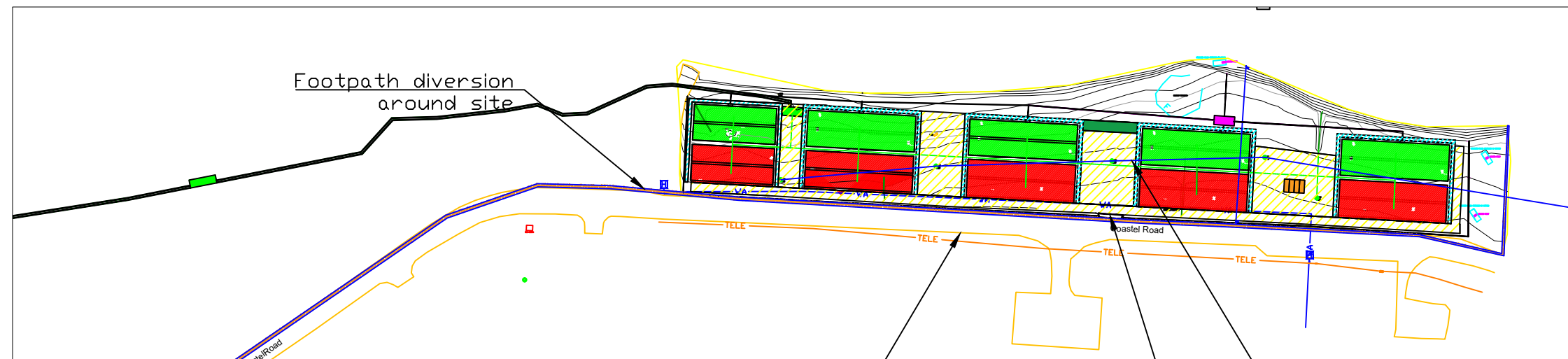
Plan showing the pumping line and Geotube layout 1:2500
