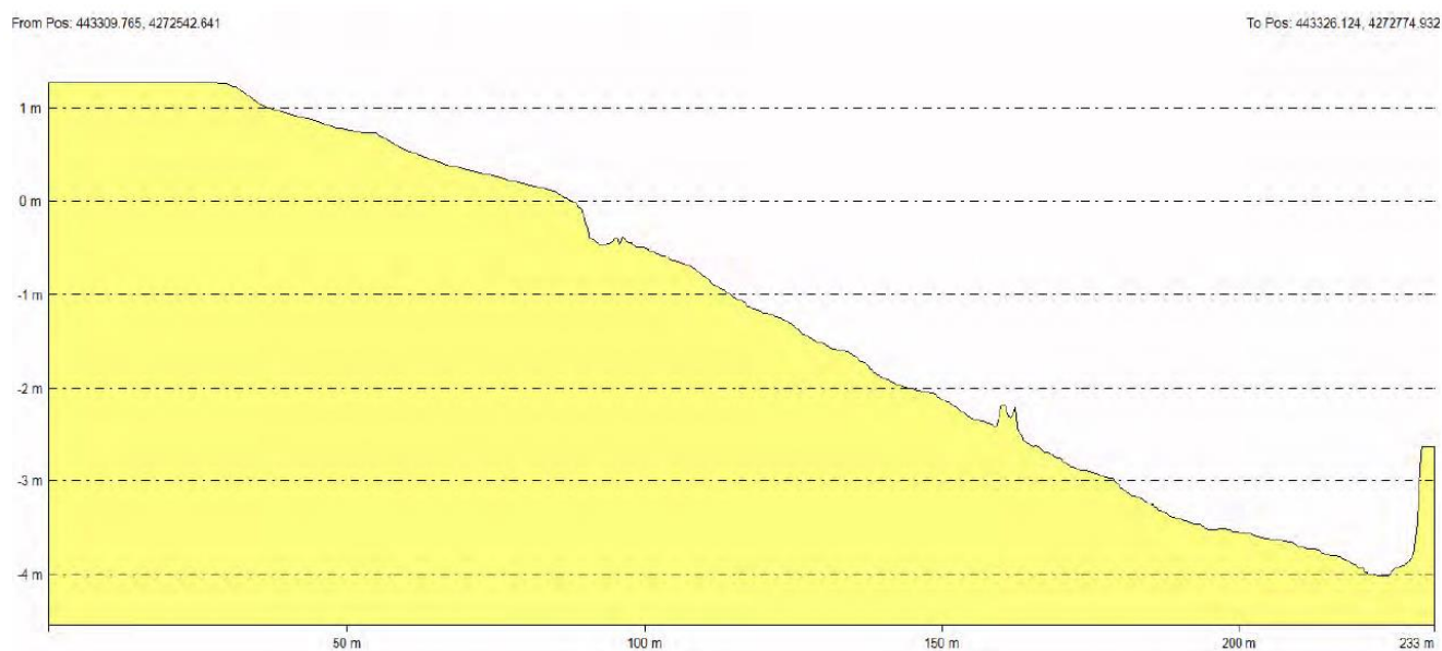
Figure 7.3 Bathymetric cross section in the vicinity of FIPASS and the proposed scheme (cross section 3 shown on Figure 7.2)
