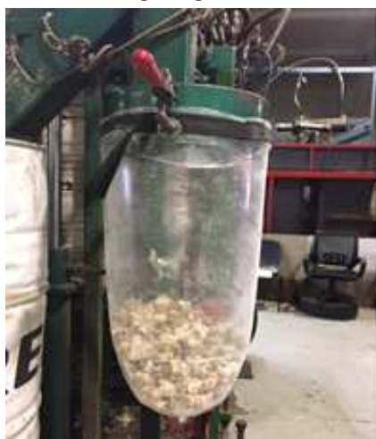
Vacuum bag taking the air pressure from the core/grab machine
