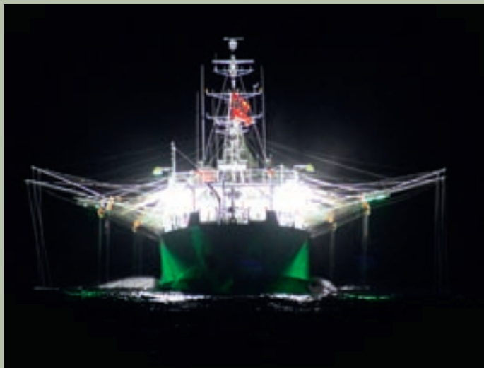
The nets of trawlers fishing for Patagonian squid are installed with Seal Exclusion Devices to protect these marine mammals.
