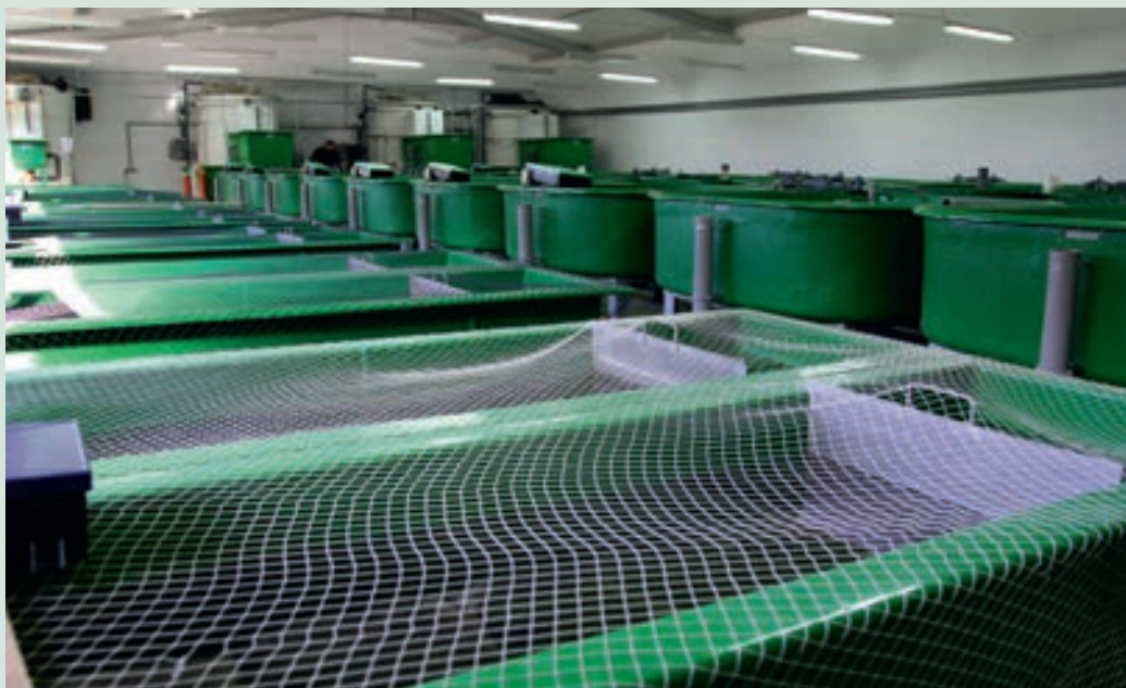
One of the most important innovations in aquaculture is the recirculating aquaculture system (RAS) which reuses the water after carefully filtering it for impurities.
